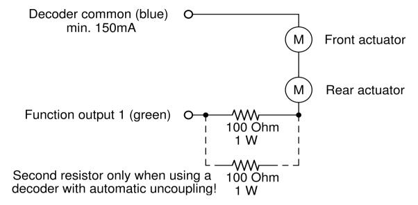
The second (paralleled) resistor has the effect that more current (250mA) is flowing through the actuators. This improves uncoupling of a single car because the opening coupler has an "kick-off" effect. Use ONLY with a properly timed decoder (ZIMO, ESU) with automatic uncoupling function, otherwise you will burn the actuators very quickly! The output must be able to supply 250 mA for a short duration.
